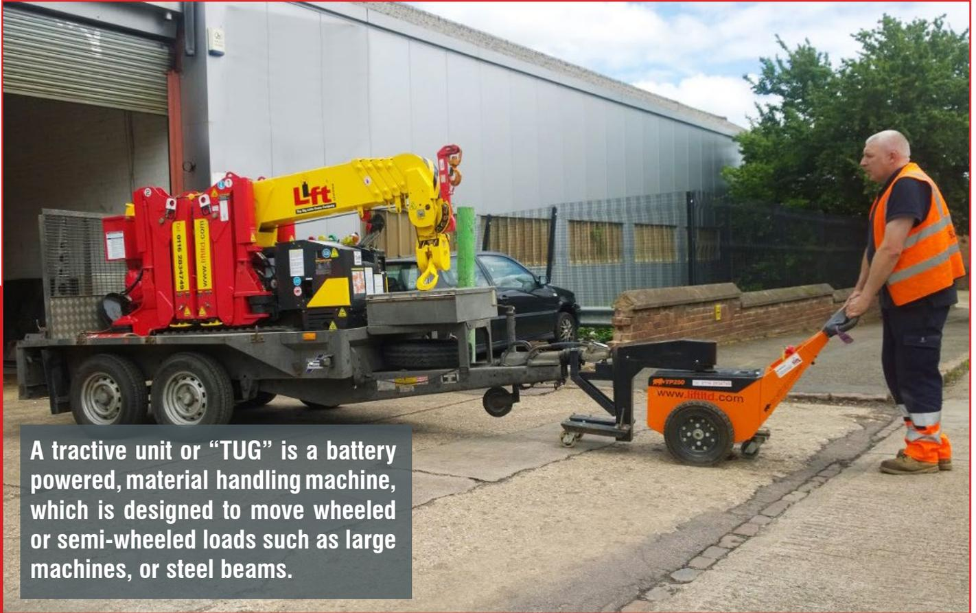
A tractive unit or "TUG" is a battery powered, material handling machine, which is designed to move wheeled or semi-wheeled loads such as large machines, or steel beams.
