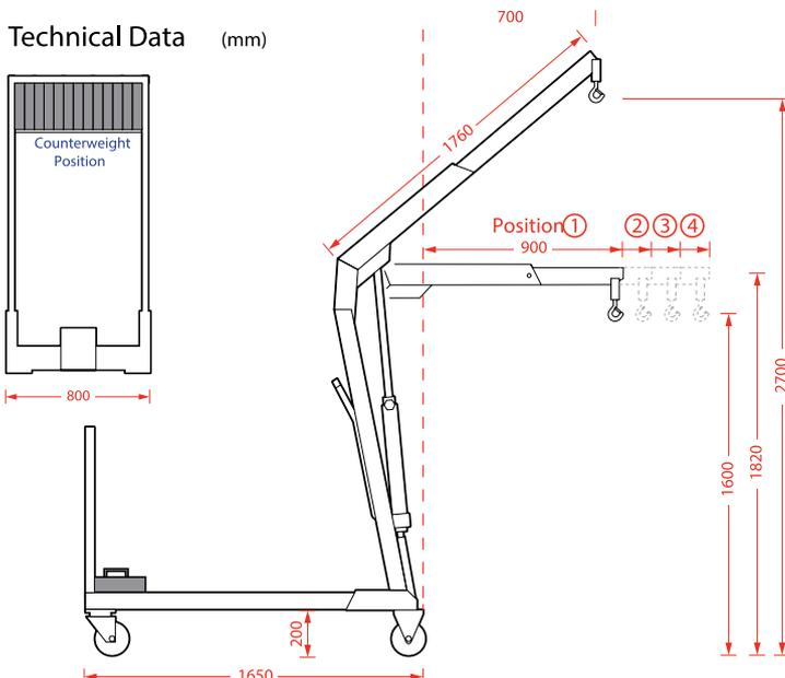
Note: Weights must be secured before lifting
